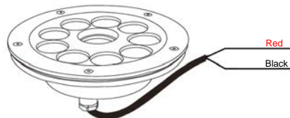
Cable connection for White
