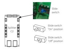
\*\*  $120\Omega$  termination switch must be on "Off" position for the last DMX splitter of the last LEDPDS panel in DMX network.
