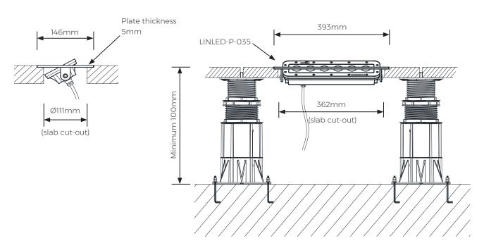
Linear LED Light LINLED Series Model No. LINLED Rev. 2
