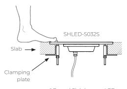
\* Round Slab hanger LED light with clamping plate for elevated floor slab installation
