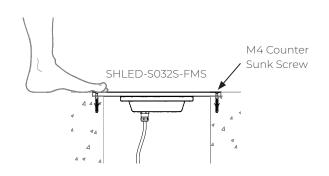
\* Round Slab hanger LED light with 2pcs-M4 counter sunk screws -for Niched installation
