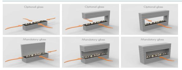
The glass shield is available on request and can be mounted on the furniture/wall in which the fire place is installed. Please see above the situation where the glass is optional and where it is mandatory.
