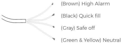
Water Level Tube Sensor Electrode Cable Connection set-up for Pools:
