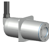
PZA-WC-NG + PZA-FLEX-S * Niche for SLP-DVM Built-in length: 262 mm Hole size: 1.5" BSP Conduit connection: 3/4" BSP
