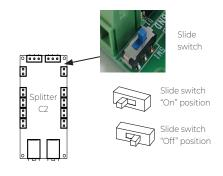
$^{**}$  120  $\Omega$  termination switch must be on "Off" position for the last DMX splitter of the last LEDPDS panel in DMX network.
